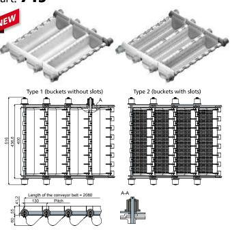
MATERIALS: Buckets and side panels in polypropylene, white colour; pins, connecting rods and split pins in stainless steel AISI 304; rollers in polyamide.
