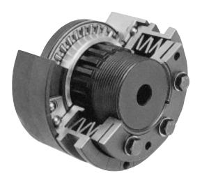
The Safegard CSF Clutch uses a large number of equally spaced balls to provide the drive, and the clutch ratchets from one drive position to the next in the event of an overload. The design allows for high operating speeds, and the possibility to recapture drive in the event of an inertia created overload during starting, but do not provide any synchronisation between input and output.
