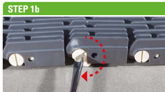
1b - Pin-clip rotated 90°.
