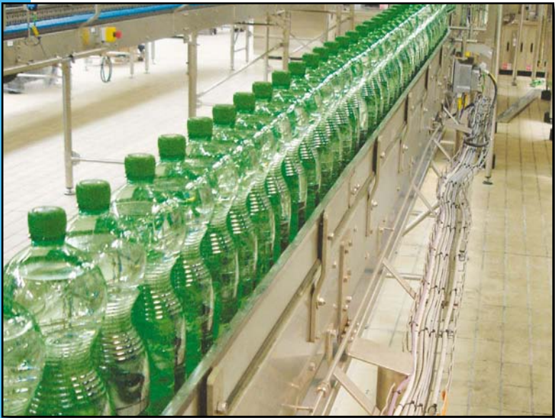
SINGLE TRACK CONVEYOR FOR PET BOTTLES.
