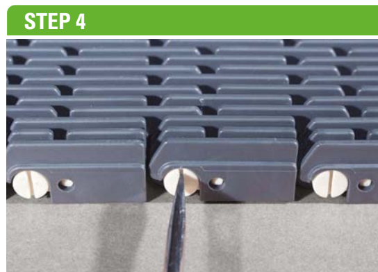
4 - Clip completely rotated. The belt is now closed.
