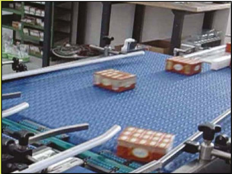
ROLLER TOP BELTS IN SORTING/POSITIONING SYSTEM.
