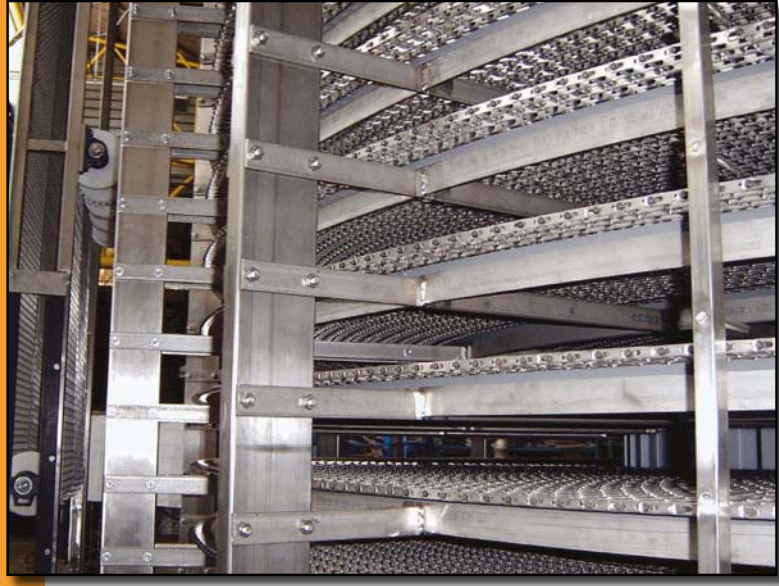
BAR CAP PROFILES FOR SPIRAL CONVEYOR SYSTEMS.
