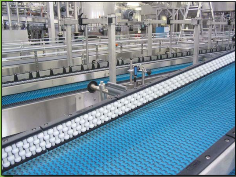
RUBBER TOP MODULAR BELTS WITH ROLLER SIDE GUIDES.
