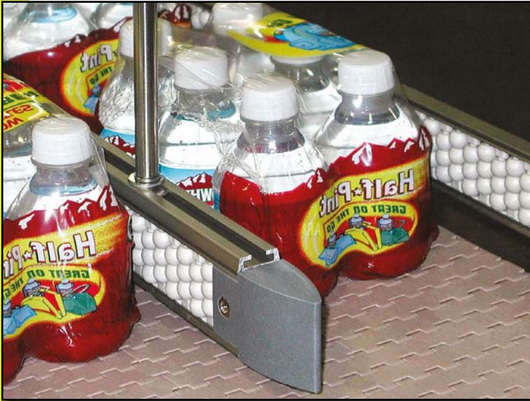
SPEEDRAIL™ ROLLER GUIDES FOR SHRINK WRAPPED PRODUCTS.
