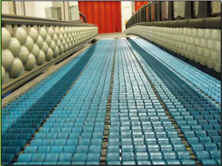
ACCUMULATION SYSTEM FOR SHRINK WRAPPED PRODUCTS.
