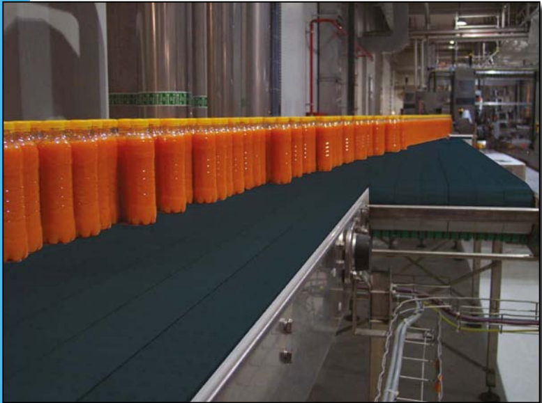
MASS FLOW TO SINGLE ROW USING 2250 MODULAR BELT.
