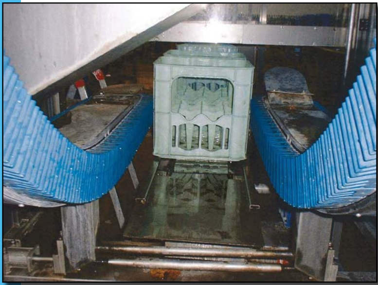
GRIPPER CHAINS FOR CRATE ELEVATORS.
