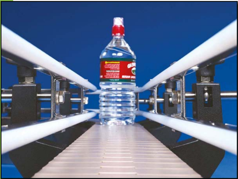
SINGLE LINE CONVEYOR SYSTEM WITH SANITARY SIDE GUIDES.
